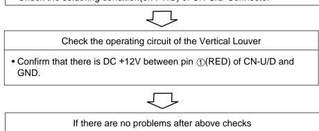
• Confirm the assembly conditions that are catching and interfering parts in the rotation radial of the Vertical Louver
